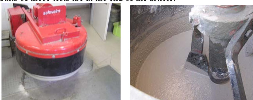
Pic. 2 Free fall concrete mixer, mixture with polypropylene fibres
