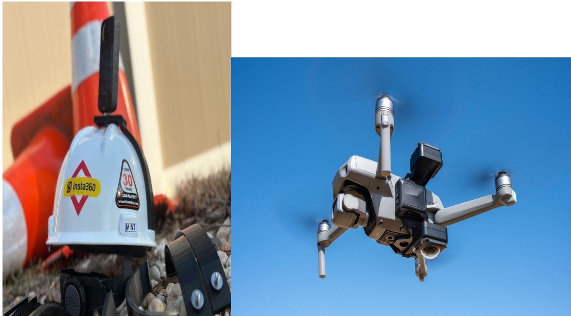
Figures 3 and 4. 360 cameras attached to a hardhat and a DJI Air 2s drone
