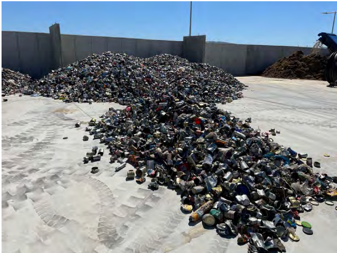
Figure 4: Separated fraction of aluminum from mixed municipal waste during the trial work on CWMC Bikarac
